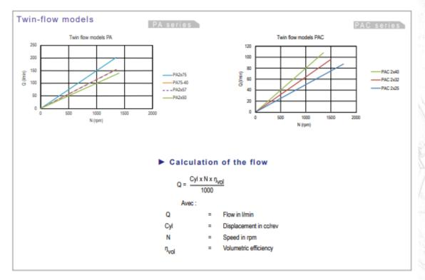
These graphs are the results of testwork done in HYDRO LEDUC R&D laboratory, on a specific test bench with a mineral hydraulic fluid ISO VG46 at 25°C (~100 cSt) - disregarding the volumetric efficiency. Volumetric efficiency
